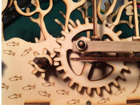
Slide block onto pins, slot in link faces shaft 2. Small washer and O-ring over pins.
