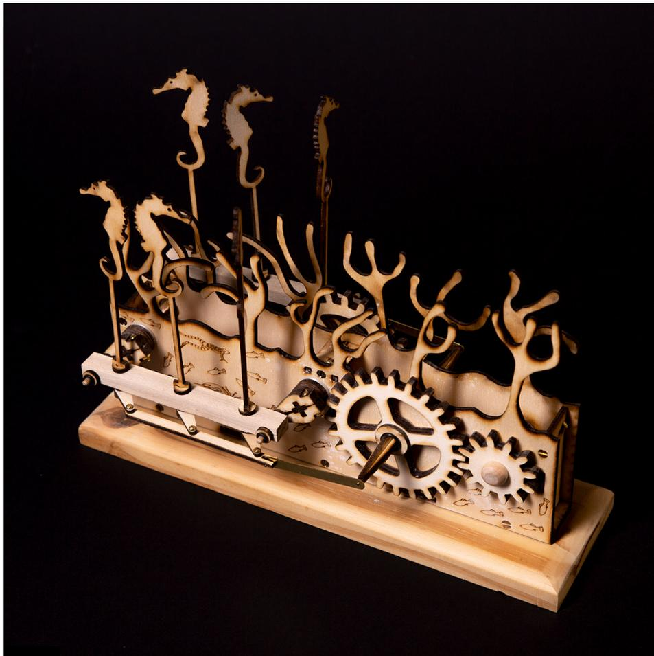
Crank your kit and look at the action. If it's tight, make sure to use the talcum powder. If it's still tight, check each shaft to see if perhaps any were squeezed too tightly during assembly and may need to be loosen up a bit.
