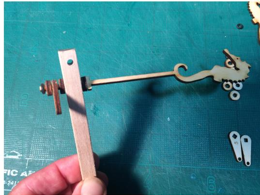
Take a **seahorse figure** and slide a **small wooden washer** up to the stop. Then insert the bottom of the seahorse stick into the wooden block. Follow that up with a **small wooden washer, a control horn, a small wooden washer, an O-ring**. Slide the O-ring on with your fingers. Populate the other two location with seahorses using the same construction technique.
