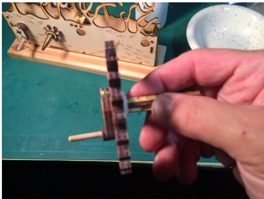
Shaft 3, crank, 24T gear, flanged washer
