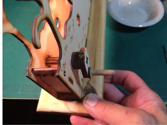
12-tooth gear, nylon flanged washer      flanged washer, 3 cross washers, handle
