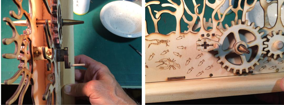
Shaft 3: nylon flanged washer, 3 cross-washers, crank.
