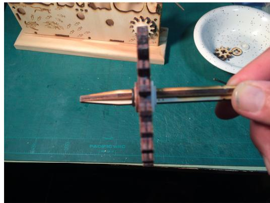
Shaft 2, Slide on the O-ring, cross-washer, 24-tooth gear, nylon flanged washer.
